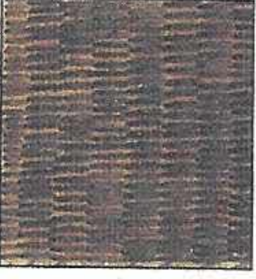
Flat shader: toe pushed in, row-next-to- row pattern
