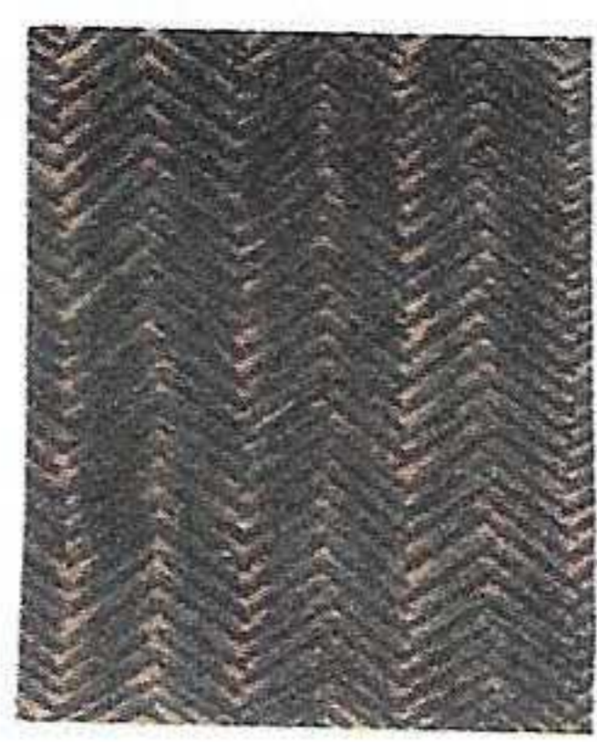
Skew: pushed in, herringbone pattern
