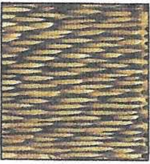
Writing nib: coolish, deep strokes, surface then burnt with shaver
