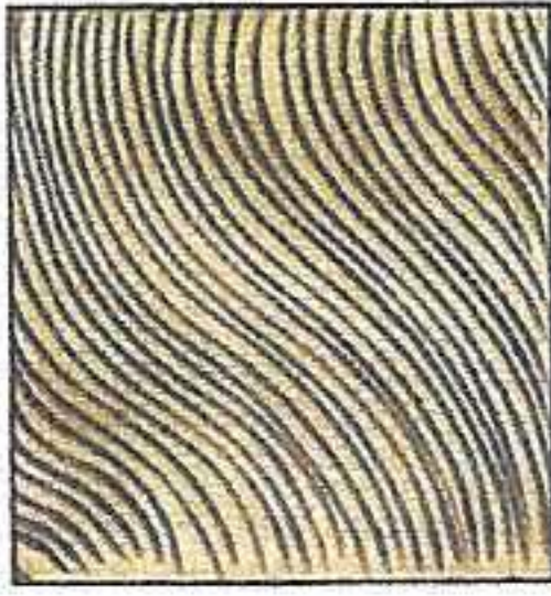
Skew: toe pushed in tight, random pattern at cross angles
