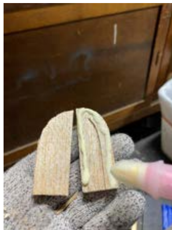
Left: Both scabbard halves with the blade pocket cut into one half. Center: applying the wood glue. Right: Clamping together.
