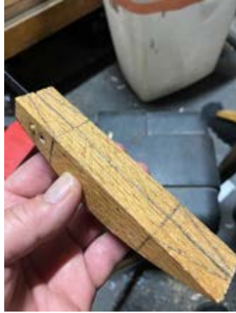
Left: Centerline and taper lines drawn on belly of handle. Center: Center line and taper lines drawn on back of handle. Right: Tapers boiled in.
