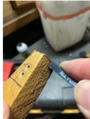
Left: rivet holes drilled and back of tang marked. Center: Cutting the kerf for the tang. Right: Cleaning out the kerf with the blade blank.
