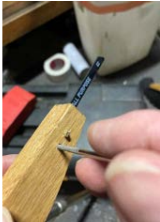
Left: Blade fitted into handle and first rivet test fitted. Center: Cleaning rivet hole before test fitting. Right: Rivets and blade blank successfully fitted to handle
