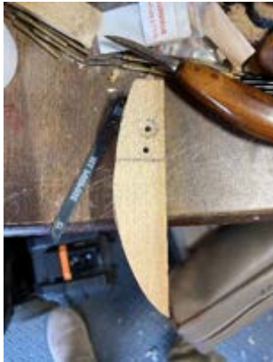
Left: rivet holes drilled and back of tang marked. Center: Cutting the kerf for the tang. Right: Cleaning out the kerf with the blade blank.
