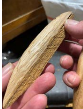
Left: Rounding the handle from centerline out to side. Center: One half of handle rounded in. Right: Handle completely rounded in.
