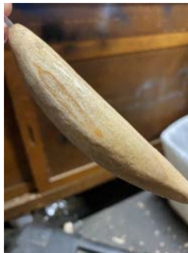
Left: Applying Cyano-Acrylate glue finish to the handle. Right: Handle completely coated with first coat of glue.
