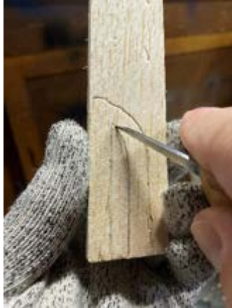
Left: Scabbard marked on a piece of 1/4" balsa wood, and stop cutting the outline of the back of the blade. Center: Shaving from the blade edge line to the stop cut. Right: Checking the flat fit.
