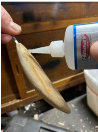
Left: Applying Cyano-Acrylate glue finish to the handle. Right: Handle completely coated with first coat of glue.
