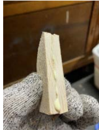
Left: Both scabbard halves with the blade pocket cut into one half. Center: applying the wood glue. Right: Clamping together.
