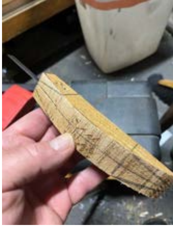
Left: Centerline and taper lines drawn on belly of handle. Center: Center line and taper lines drawn on back of handle. Right: Tapers boiled in.
