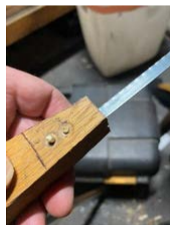
Left: Blade fitted into handle and first rivet test fitted. Center: Cleaning rivet hole before test fitting. Right: Rivets and blade blank successfully fitted to handle
