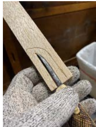
Left: Scabbard marked on a piece of 1/4" balsa wood, and stop cutting the outline of the back of the blade. Center: Shaving from the blade edge line to the stop cut. Right: Checking the flat fit.
