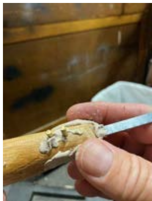
Above: Blade pushed in and rivets installed. Notice that the putty completely covers all parts of the kerf.
