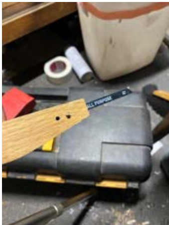
Left: Blade fitted into handle and first rivet test fitted. Center: Cleaning rivet hole before test fitting. Right: Rivets and blade blank successfully fitted to handle
