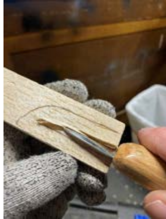
Left: Scabbard marked on a piece of 1/4" balsa wood, and stop cutting the outline of the back of the blade. Center: Shaving from the blade edge line to the stop cut. Right: Checking the flat fit.
