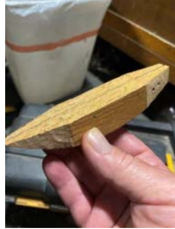
Left: Centerline and taper lines drawn on belly of handle. Center: Center line and taper lines drawn on back of handle. Right: Tapers boiled in.
