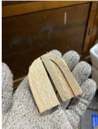
Left: Both scabbard halves with the blade pocket cut into one half. Center: applying the wood glue. Right: Clamping together.
