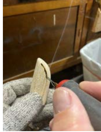
Left: Rounding the scabbard. Center: Scabbard rough carved and ready for sanding. Right: After sanding, burning in flat diamond gripping surface to match knife handle.
